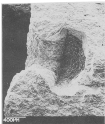
Fig. 6. SEM photograph of a \beta -PbO 2 layer (removed from a \beta -PbO 2 (Ti) electrode) parallel to the growth direction. The substrate (titanium) is towards the right side of the figure.
